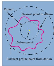
**↗ = Runout (Runout)**
